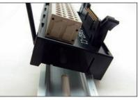
1. Insert a flat-blade screwdriver into the DIN Track lock. 2. Move the screwdriver like a lever to free the lock.
