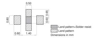
\* Make sure to connect the GND terminal of this product and the GND of the mounting circuit board by using through holes so that the distance between them is the shortest.
