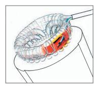
• PTC's are classified according to their nominal response temperature  $\delta_{\text{NAT}}$  but all have similar resistance characteristics to simplify the choice of switching device; the relationship of resistance to temperature of all these PTC's is as follows:
