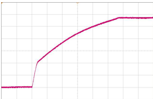
Figure 9. Turn-On AC Line 230 VAC, full load (2 ms/div) CH4: V SB (2 V/div)
