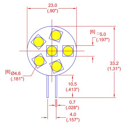
NOTE: OVERALL THICKNESS OF ASSEMBLY IS LESS THAN 10mm (.394").
