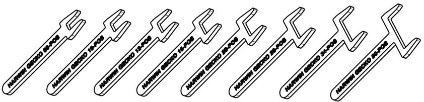
TOOLS TO BE USED FOR DELATCHING G125-SERIES CONNECTORS.
