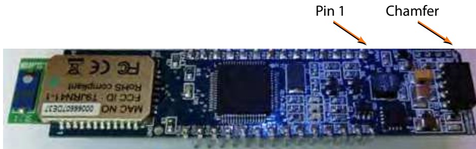
Figure 2. The Location of Pin 1 and Chamfer on the Mini-Z Z-PAN® 28-Pin Module
