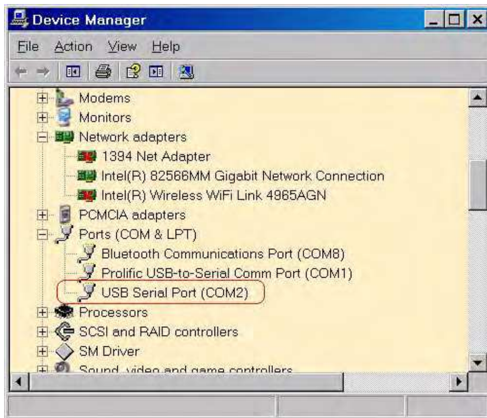
Figure 11. A Successful USB-to-UART Driver Installation
