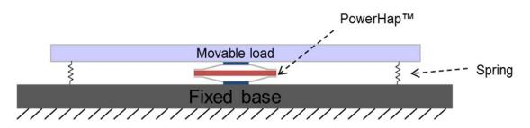
By applying a voltage to the actuator, it elongates and therefore moves the load. This movement can be felt by the user. For a maximal haptic feedback, the rear panel needs to be as heavy as possible. Otherwise the PowerHap actuator will not only move the load but also the rear panel and therefore a part of the performance is lost.
