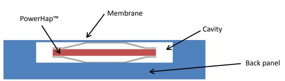
In this case the PowerHap actuator is clamped between a thin, flexible membrane and a rigid back panel. By applying a voltage, the actuator elongates and consequently deforms the membrane.
