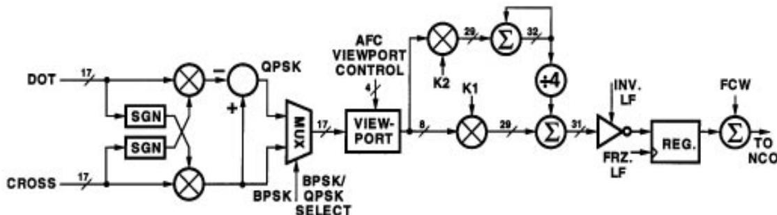
Figure 9. Frequency Discriminator and Loop Filter Detail
