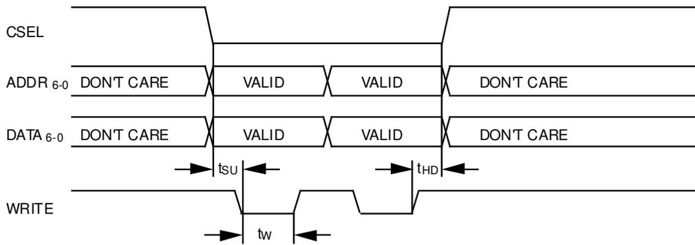
Figure 3. Microprocessor Interface Timing
