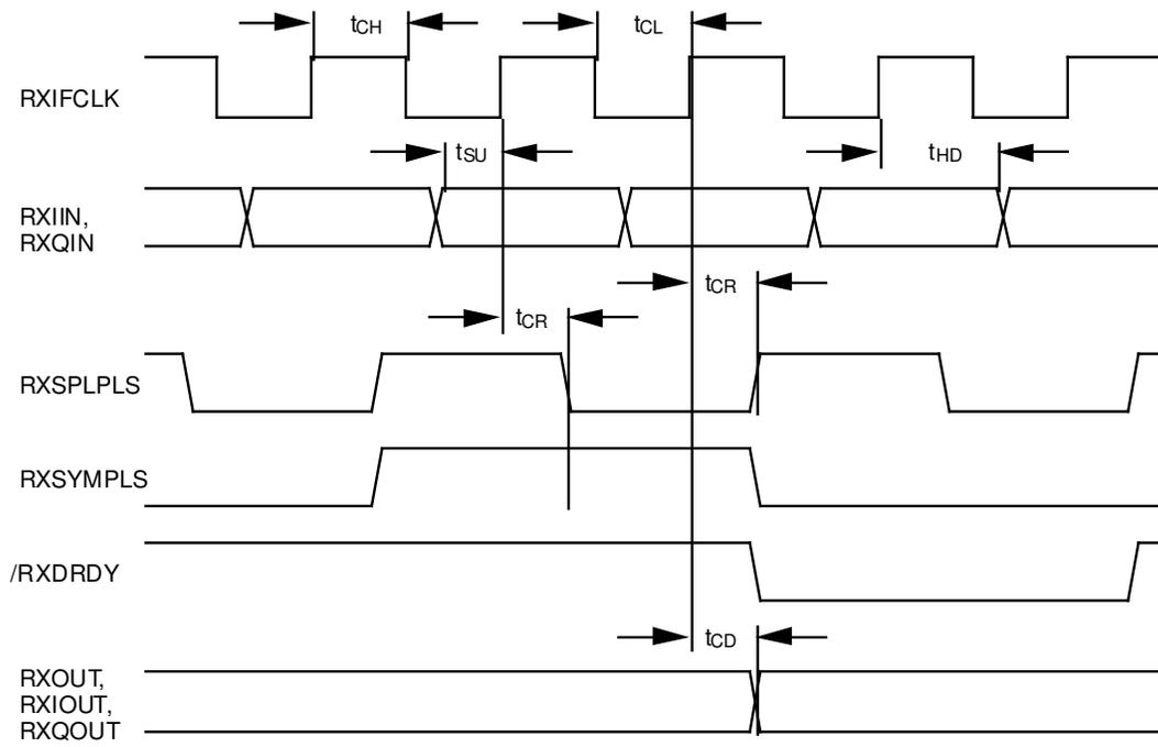
Figure 5. Receiver Input/Output
