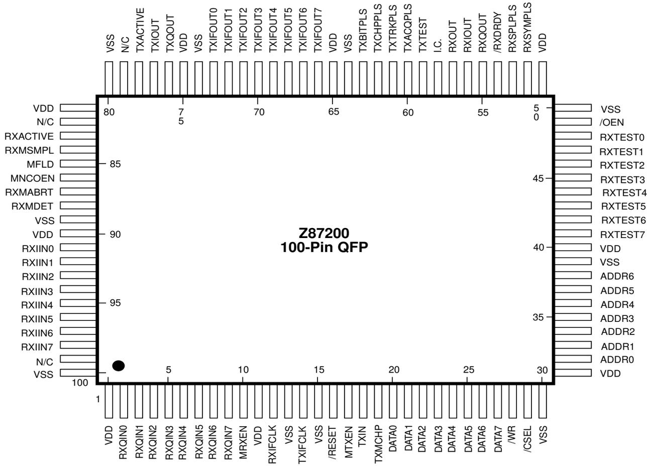
**Figure 2. Z87200 100-Pin PQFP Pin Description**
