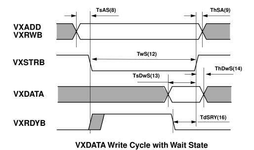
Figure 9. Read/Write Cycle Timing with Wait StatE
