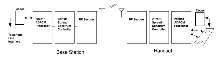
Figure 1. System Block Diagram of a Z87001/Z87010 Based Phone
