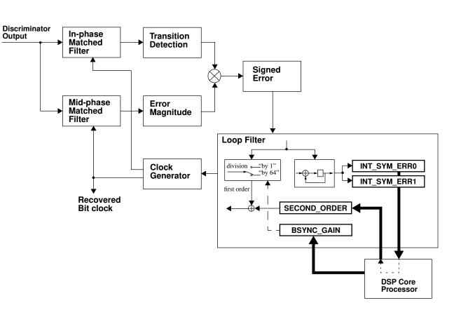
Figure 6. Bit Synchronizer Loop and Processor Control
