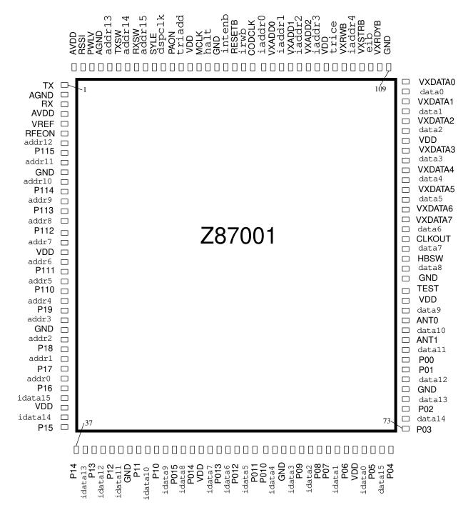
Figure 3. 144 Pin QFP Pin Configuration
