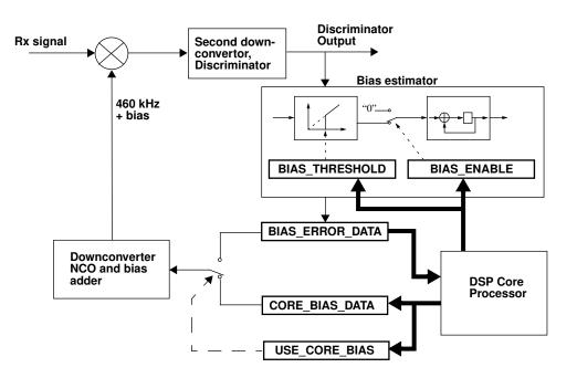
Figure 5. AFC Loop and Processor Control
