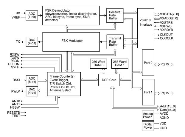
Figure 2. Z87001 Functional Block Diagram
