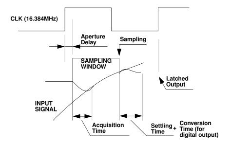
Figure 6. 1-Bit ADC Definition of Terms
