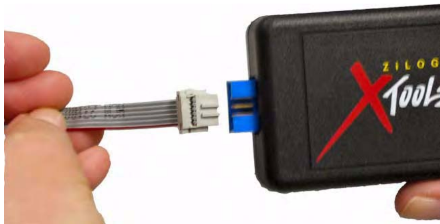
Figure 3. Connecting the 6-Circuit Ribbon Cable to the USB SmartCable
