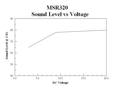
For audible alarm model MSR320R, the sound level will vary from 65 dB at 2 ft. at 3 Vdc up to 80 dB at 2 ft. at 20 Vdc. By varying the voltage from 3 to 20 Vdc, the sound level can be varied by 15 dB. A 10 dB drop in sound level will make the alarm sound half as loud.
