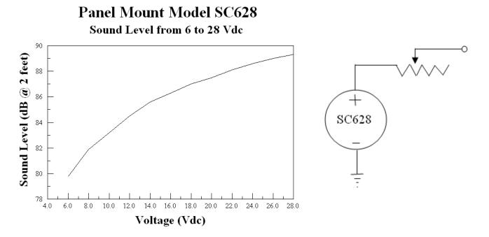
It was verified that the circuitry of model SC628R is not affected by a potentiometer, so data was gathered to find the value of a potentiometer that gives the greatest range of sound change.
