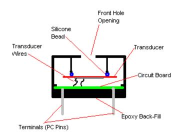
Piezoelectric Audible Signal Basic Construction
