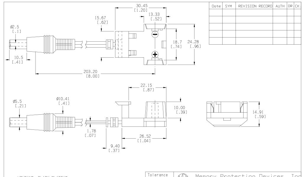
HOUSING: BLACK PLASTIC CORD: UL2468, 300V, 80°C, 22-24AWG PASSES UL FLAME TEST VW-1 FILE NO. E11278 OR EQUAL CENTER IS POSITIVE CONTACT DC MOLDED PLUG: 2.5mm X 5.5mm
