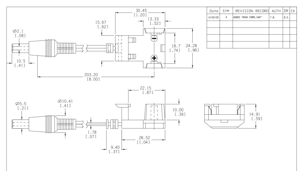
HOUSING: BLACK PLASTIC CORD: UL2468, 300V, 80°C, 22-24AWG PASSES UL FLAME TEST VW-1 FILE NO. E11278 OR EQUAL CENTER IS POSITIVE CONTACT DC MOLDED PLUG:2.1mm X 5.5mm FOR 2.5mm X 5.5mm USE P/N ZA5350-2.5 ROHS COMPLIANT
