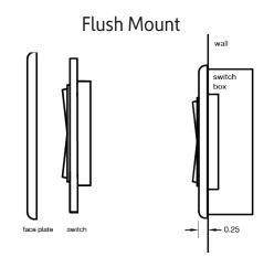
For flush mount, mount the switch without the backplate into either a standard electrical switch box or a low voltage mounting bracket using included screws.
