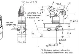
One-way Action Sealed Roller Arm Lever
