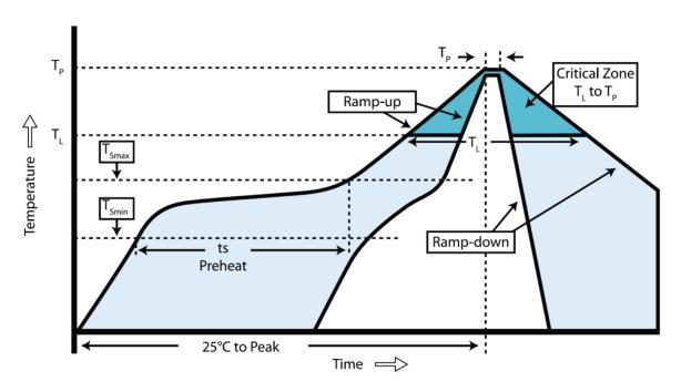
ZETA is a 2 layer PCB, re-flow is based on IPC/JEDEC JSTD020C July 2004
