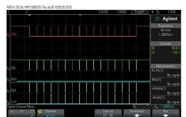
Above is the complete SPI & IRQ Timing diagram for #R<RSSI> <Packet > plus 12 byte data packet
