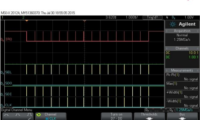
Above is the complete SPI & IRQ Timing diagram for #R<RSSI> <Packet > plus 12 byte data packet
