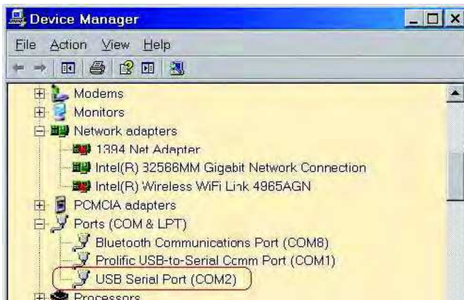
Figure 2. A Successful USB-to-UART Driver Installation
