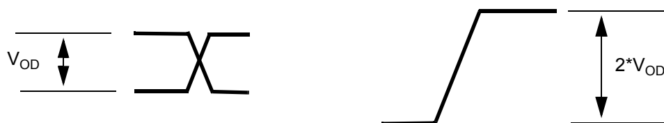
Figure 19 - Differential Output Voltage Parameter
