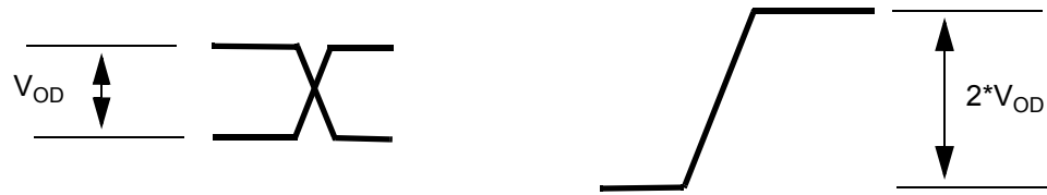
Figure 19 - Differential Voltage Parameter
