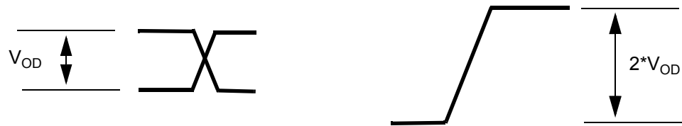
Figure 19 - Differential Voltage Parameter
