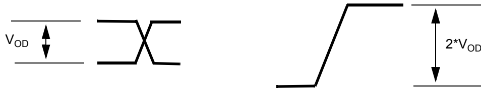
Figure 19 - Differential Output Voltage Parameter
