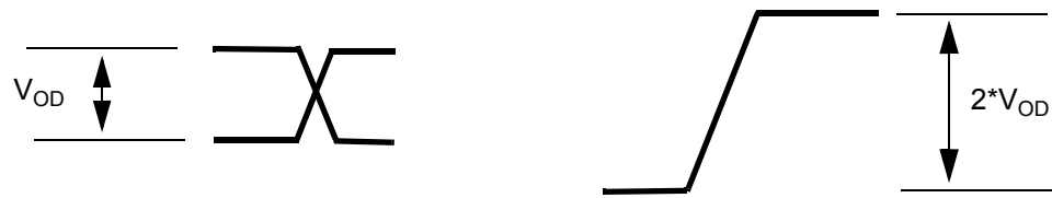
Figure 20 - Differential Voltage Parameter
