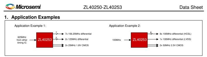
Figure 2 - Application Examples: Ethernet and PCIe Clocks
