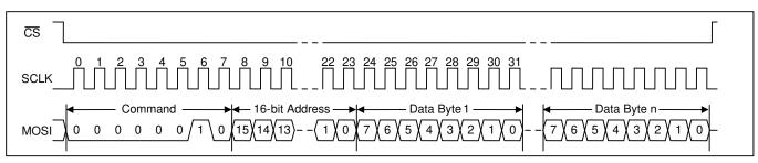
Figure 7 - SPI Write Transaction Functional Timing
