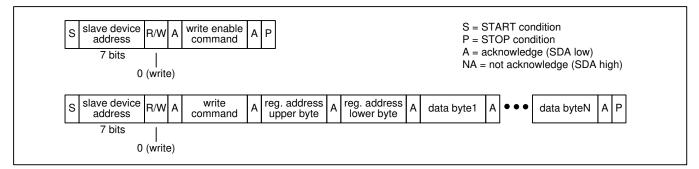
Figure 10 - I<sup>2</sup>C EEPROM Write Transaction Functional Timing (ZL40251 and ZL40253 Only)
