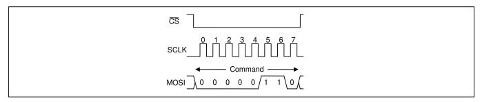
Figure 6 - SPI Write Enable Transaction Functional Timing (ZL40251 and ZL40253 Only)
