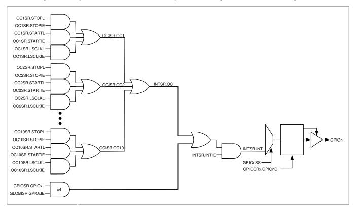
Figure 12 - Interrupt Structure
