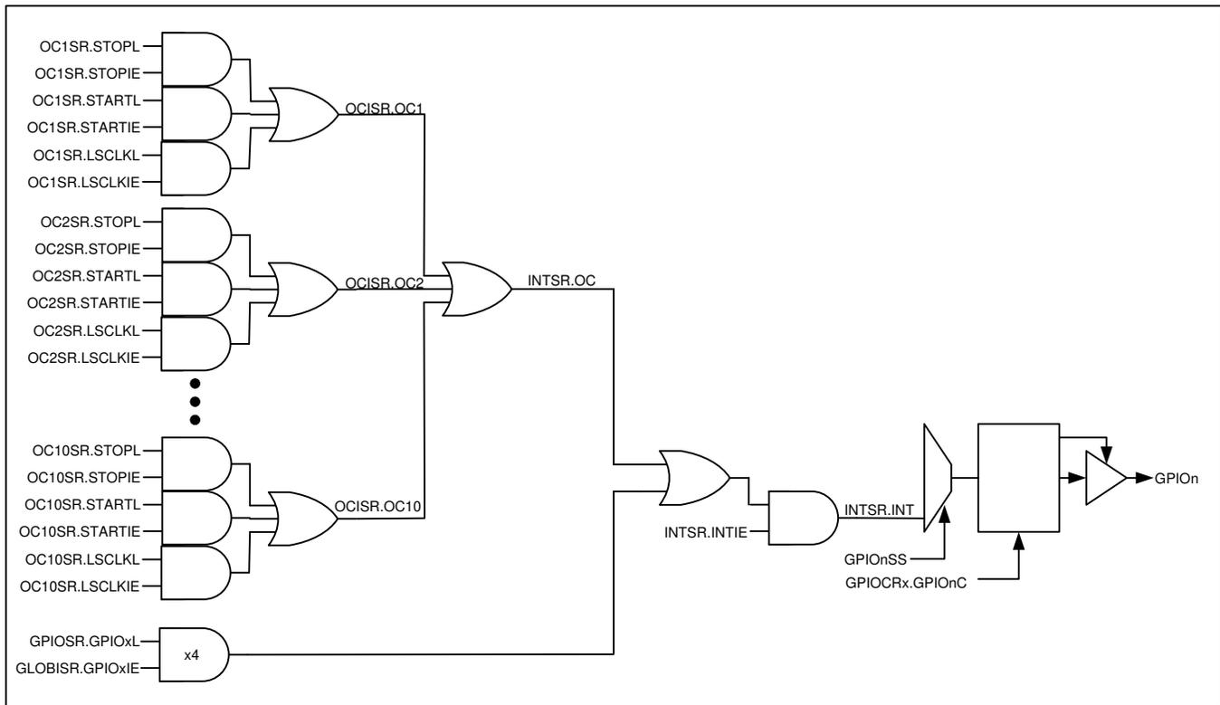
Figure 12 - Interrupt Structure
