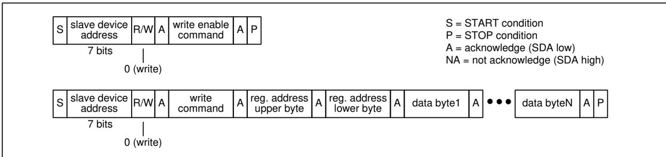
Figure 10 - I<sup>2</sup>C EEPROM Write Transaction Functional Timing (ZL40251 and ZL40253 Only)
