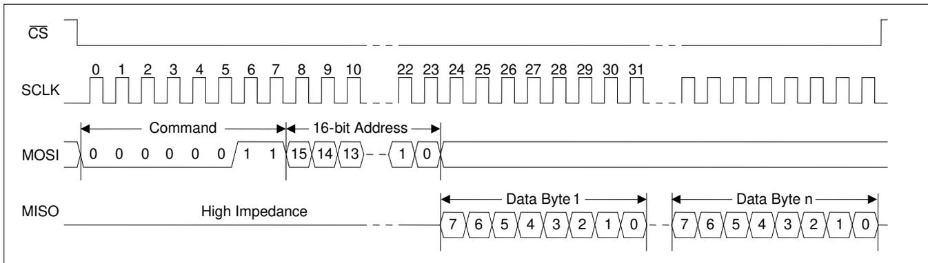
Figure 5 - SPI Read Transaction Functional Timing
