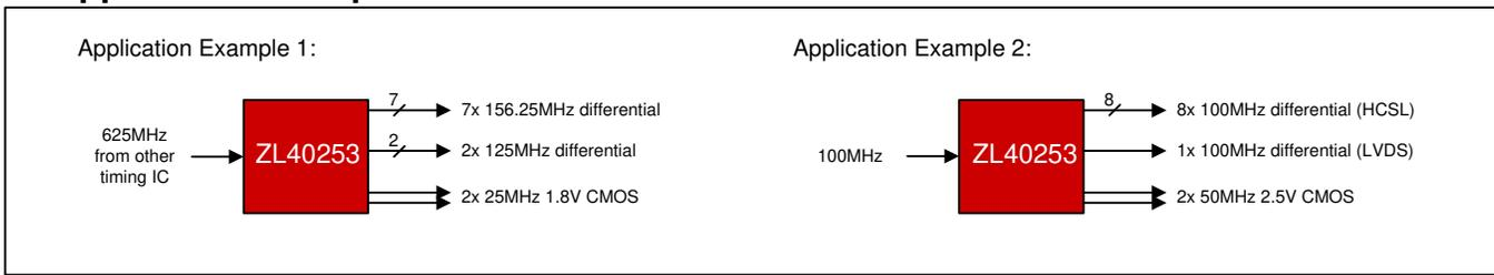
Figure 2 - Application Examples: Ethernet and PCIe Clocks
