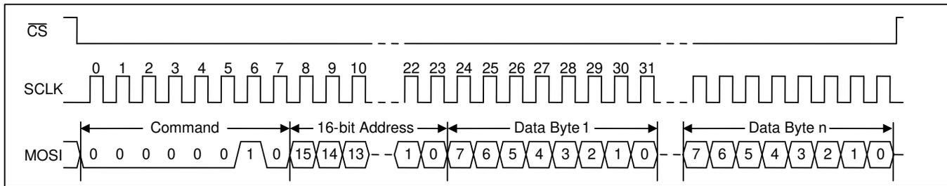
Figure 7 - SPI Write Transaction Functional Timing
