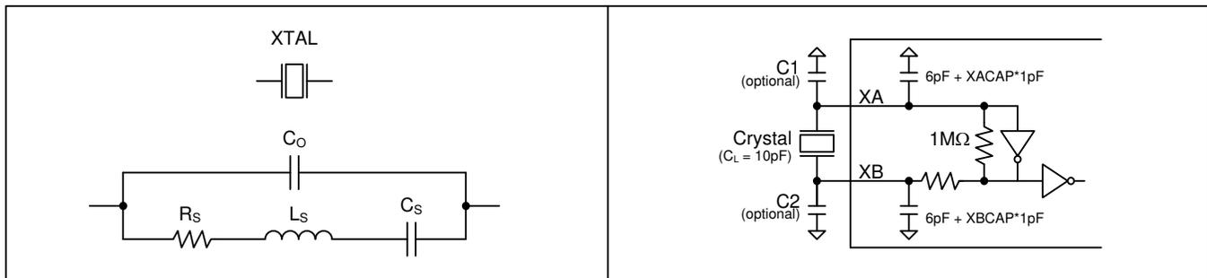
Figure 4 - Crystal Equivalent Circuit / Recommended Crystal Circuit
