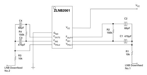
The following circuit shows the additional components that will be used for polarisation mode and 22kHz tone detection in a typical ZLNB2003/4 application.
