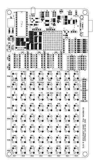
Figure 1. The ZiLOG Crimzon<sup>TM</sup> Development Board Accessory Kit
