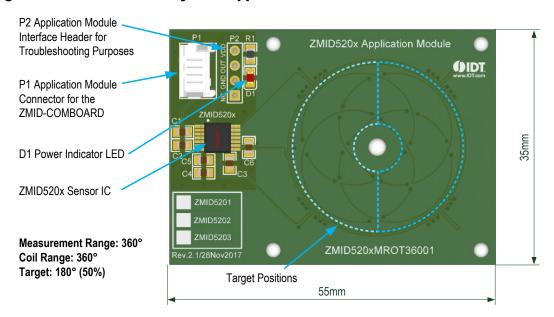
Figure 5. ZMID520x Arc 130°Application Module - Overview
