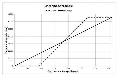
Figure 24. Modulus Output Example with Slope = 2, Offset = 60°
