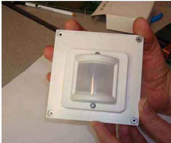
Figure 10. Assembled Flat 0.9" Lens Holder and Flat Lens
