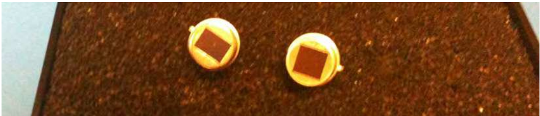
Figure 2. Two Additional Pyroelectric Sensors (L–R): SDA02-54-P and SBDI46-504AA
