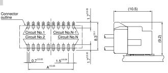
Note: 1. Tolerances are non-cumulative: ±0.05mm for all centers. 2. The dimensions above should serve as a guideline. Contact JST for details.
