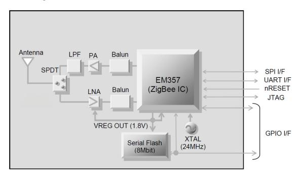
Figure 1 - ZPM3750 Module Block Diagram
