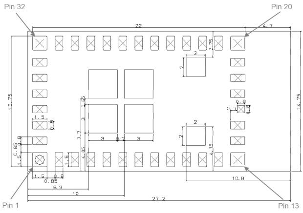
Figure 7 - Recommended Host (customer) PCB Pattern
