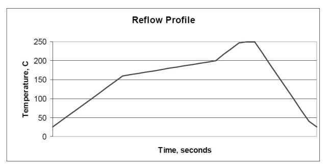
Figure 13 - Reflow Profile Pattern
