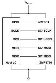
Figure 6 - SPI Host Interface Reference Diagram
