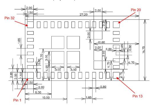
Figure 4 - Detailed Mechanical Data (top view)
