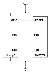
Figure 5 - UART Host Interface Reference Diagram
