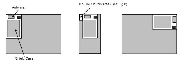
Figure 9 - Recommended Locations in x-y Plane
