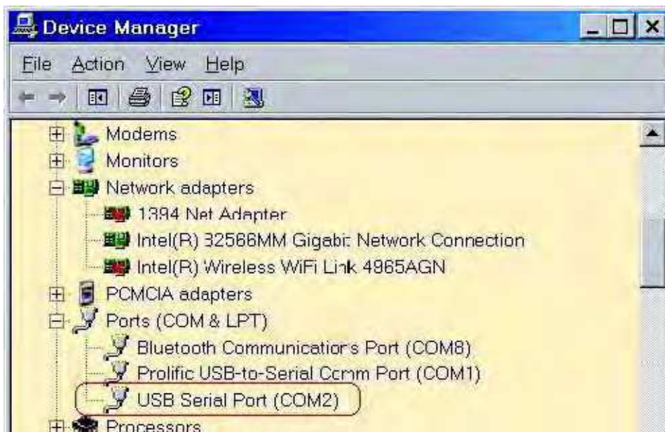
Figure 11. A Successful USB-to-UART Driver Installation
