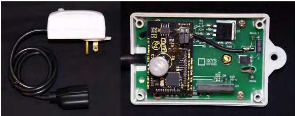
Figure 1. The Current Sensing Power Switch SCR with ZMOTION Control Reference Design with a ZMOTION Detection Module II
