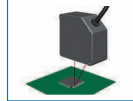
Inspecting for Board Coplanarity
