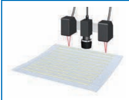
Inspecting Glass Heights (Autofocus)
