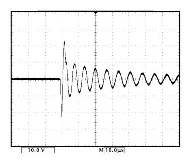
Unloaded high voltage output 10 µs/div 10 kV/div
