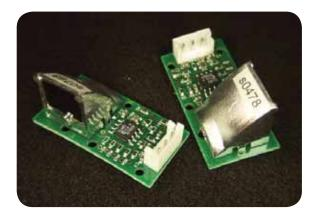
The ZTP-115M is a single IR module used for noncontact surface temperature measuring. It consists of a thermopile, IR sensor, signal conditioning and voltage output.
