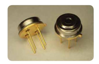
This thermopile sensor is used for non-contact surface temperature measuring. The ZTP-115 model consists of thermo-elements, flat IR filter, a thermistor for temperature compensation and a hermetically-sealed small-size package. There is also a variety of filters available to maximize performance in specific applications
