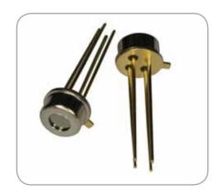
This thermopile sensor is used for non-contact surface temperature measuring. The ZTP-135BS model consists of thermo-elements, a flat IR filter, and a thermistor for temperature compensation in a hermetically-sealed TO-46 (18) package. There is also a variety of filters available to help maximize performance in specific applications.
