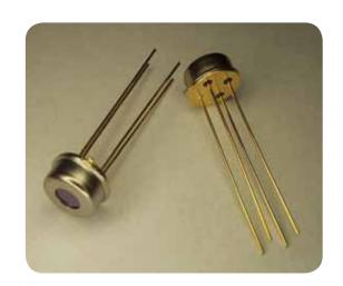
This thermopile sensor is used for non-contact surface temperature measuring. The ZTP-135L model consists of thermo-elements, flat IR filter, a thermistor for temperature compensation and a hermetically-sealed small-size package. There is also a variety of filters available to maximize performance in specific applications
