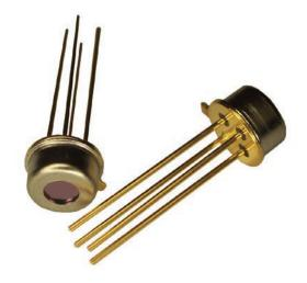
Thermometrics Thermopile IR Sensors are used for non-contact surface, or infrared, temperature measurement. The ZTP-148SR Model consists of thermo-elements, flat infrared filter and thermistor for temperature compensation, all in one hermetically-sealed TO-46 (18) sensor package. There are a variety of filters available to maximize performance in specific applications.
