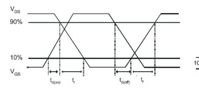
Switching Time Waveforms
