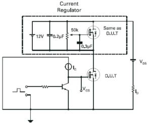
**Gate Charge Test Circuit**
