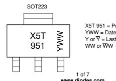
X5T 951 = Product Type Marking Code YWW = Date Code Marking Y or  $\overline{Y}$  = Last Digit of Year (ex: 5= 2015) WW or  $\overline{W}W$  = Week Code (01~53)
