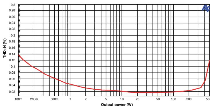
This plot shows the THD+N versus power plot for a 500W closed loop subwoofer reference design. THD+N is 0.02% between 10W and 200W which is outstanding performance.
