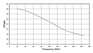
The curve shows Q Factor over frequency for a fixed loop gain (Rf/Ri).
