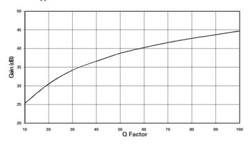
Gain at fo describes the peak gain of the notch pass filter. This gain is defined by the value of Q Factor.
