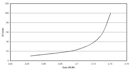
This diagram shows the exponential relationship between gain and Q Factor. (fo = 140 kHz)
