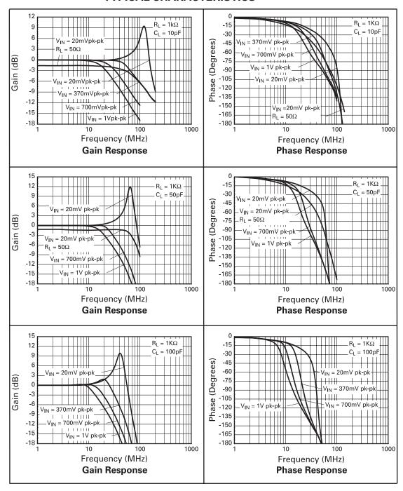
Test Conditions:V+=5V, Temperature=25°C.
