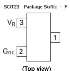
Pin 1 floating or connected to pin 2
