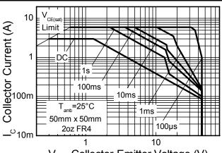
V<sub>CE</sub> Collector-Emitter Voltage (V) **Safe Operating Area**
